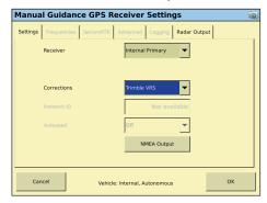
**Note:** The FmX integrated display must be unlocked for RTK to use the VRS correction type.
